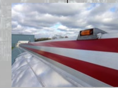
VAPOR RAIL LIGHTS
